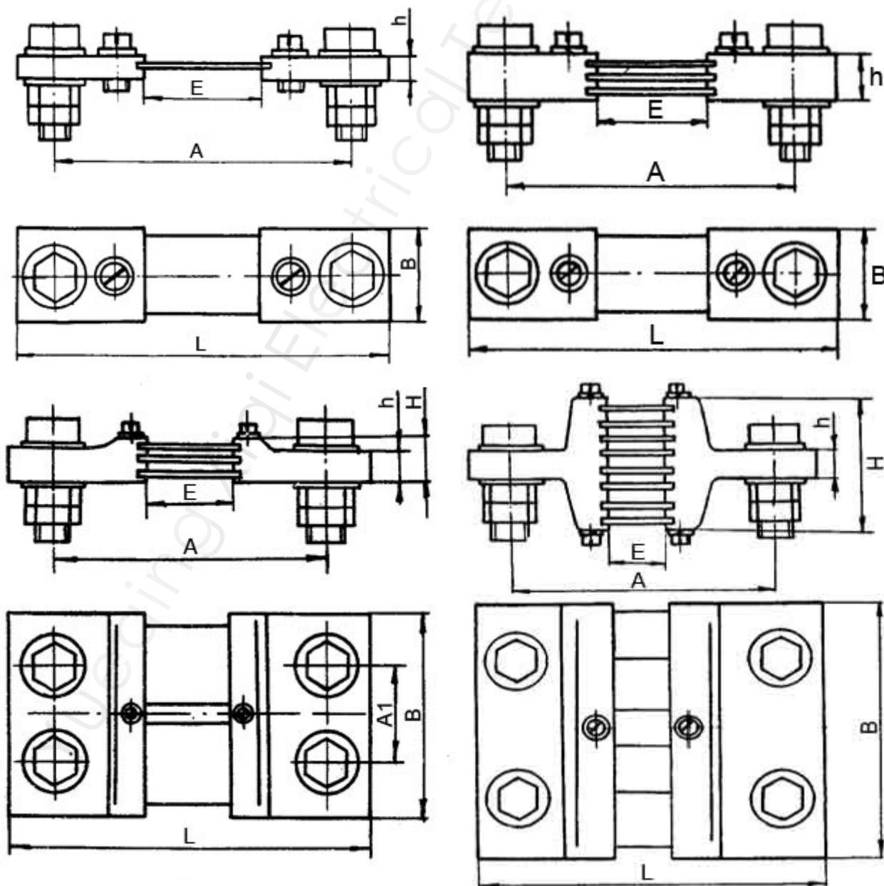
■ FL-19 Shunt(Welding Machine Type)
